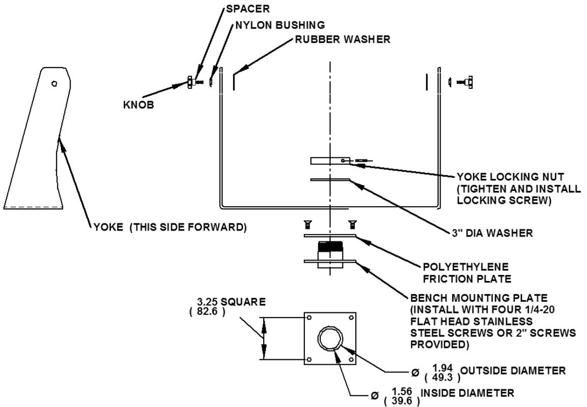
1. Insure mounting surface is smooth enough to seal with gasket and create mounting pattern in surface per the above diagram.
