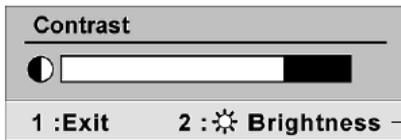
The line at the bottom of the screen shows the current functions of buttons 1 and 2: Exit or select the Brightness control.
