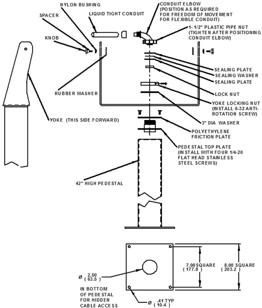
**Note:** The 3/4" conduit and other sealing hardware are not required for NEMA 12 monitors or NEMA 4/4X monitors with the 4-cable gland.
