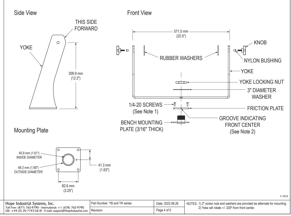
Mechanical Drawing – Yoke Mount with Benchtop Mounting Kit
