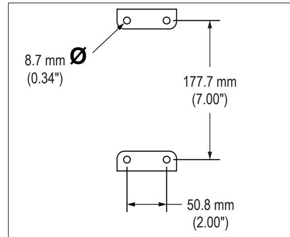
FIGURE 2 – YA \_\_ -24- \_\_ MOUNTING PATTERN
