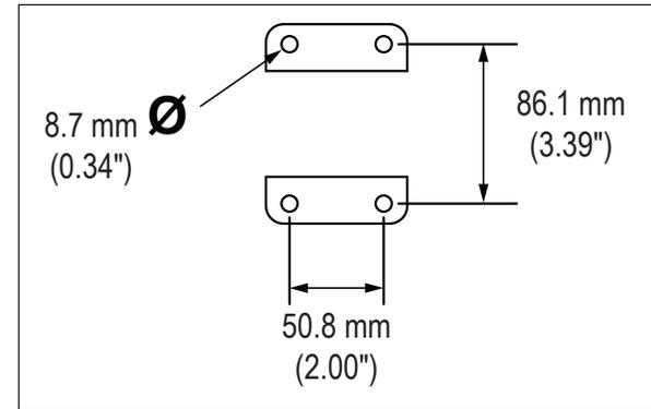
FIGURE 1 – YA \_\_ -15- \_\_ MOUNTING PATTERN
